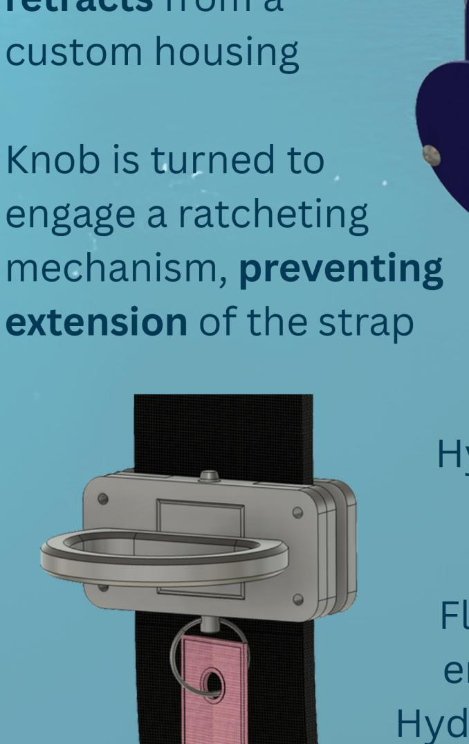
Specialized carabiner clasps onto D-ring on the diver's gear in a **simple and fast motion**
