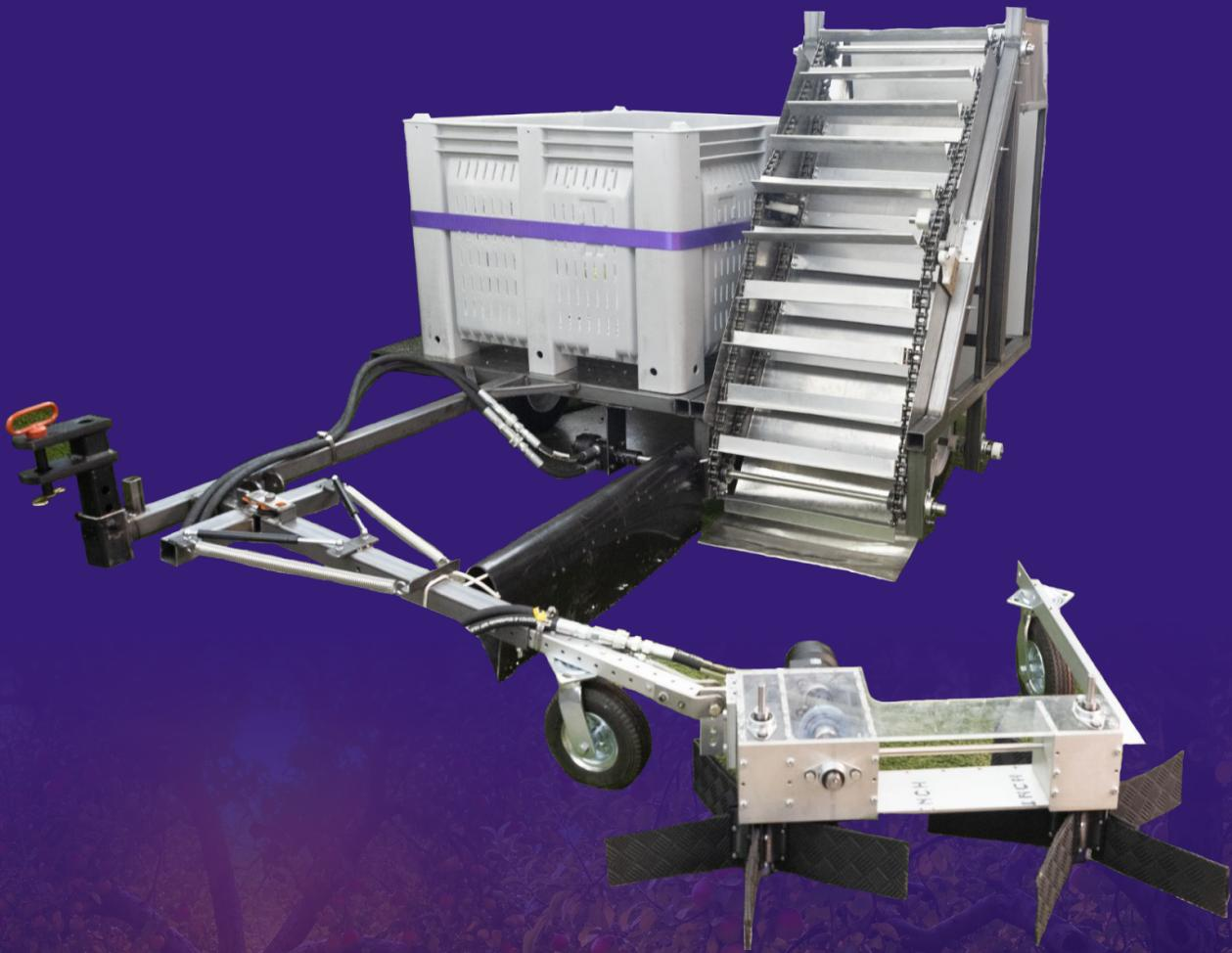
**A hydraulic-powered tractor attachment that sweeps and collects fallen apples out from beneath orchard trees**
